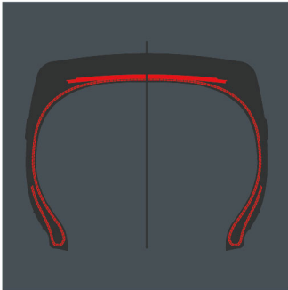
Tough casing construction for enhanced impact and cut resistance support
